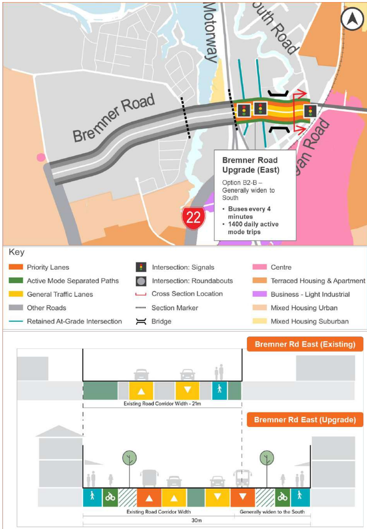
Figure 9-24 Bremner East FTN Arterial Upgrade preferred cross-section
