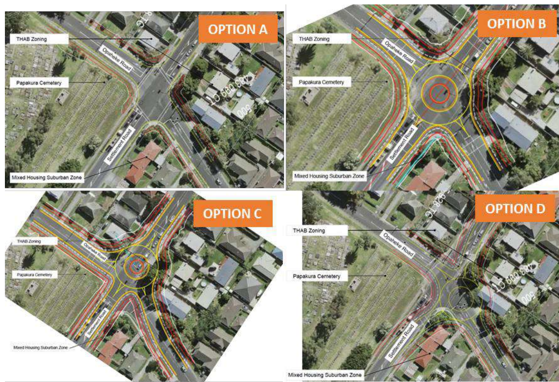
Figure 9-47 Intersection treatment options
